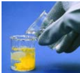
Figure 4.1 The reactants potassium iodide and lead(II) nitrate are both clear. The chemical reaction that takes place when they are combined results in a colour change in the product.
