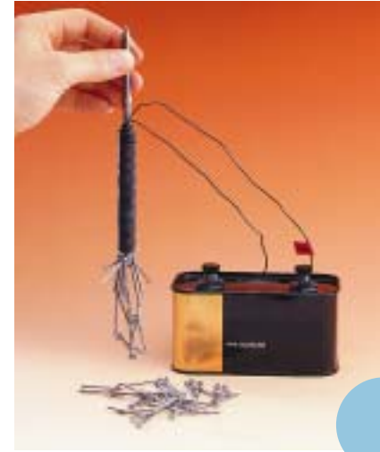
Figure 3.9 An electromagnet is made by winding a current-carrying wire around a metal core.
