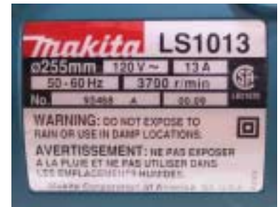
Figure 1.15 A Canadian Standards Association label listing voltage and current for an appliance
