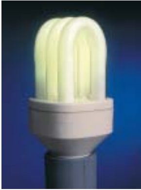
Figure 3.25 In a fluorescent tube, an arc through mercury vapour produces ultraviolet (UV) light. The tube's fluorescent coating absorbs the UV light and re-emits it as visible light.
