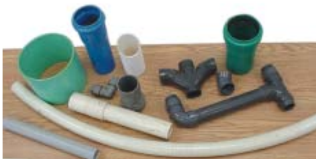
Figure 1.26 These PVC pipes and the PVC insulation on these wires are made with chlorine produced by electrolysis.
