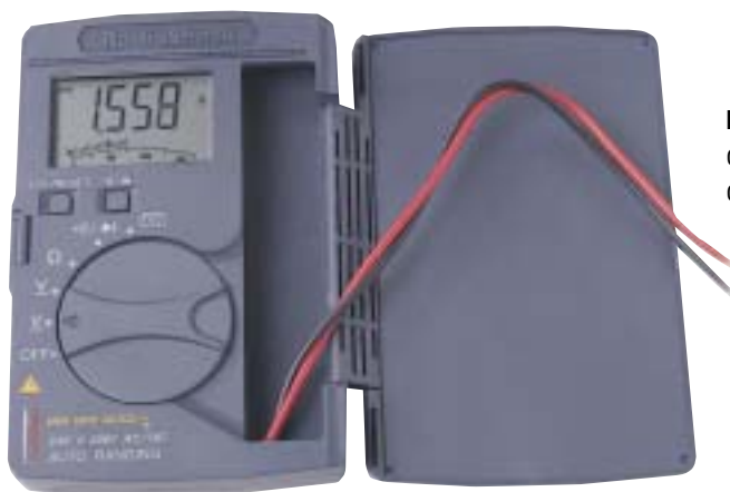
Figure 1.9 Some voltmeters have more than one range of measurement.
