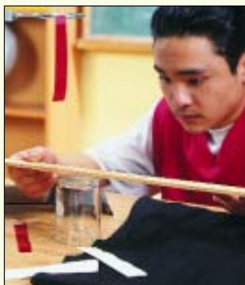
Figure 1.3 Balance the metre stick on the watchglass on top of the beaker.
