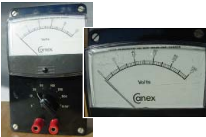
Figure 1.9 Some voltmeters have more than one range of measurement.
