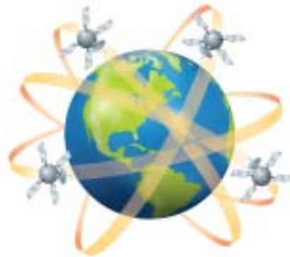
Figure 2.28 With 24 satellites in orbit, there are at least three above the horizon, relative to a person's location on Earth, at any one time.
