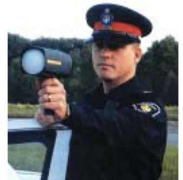
Figure 3.28 Radar guns used to enforce traffic speed limits were developed based on scientific understanding of the Doppler effect.
