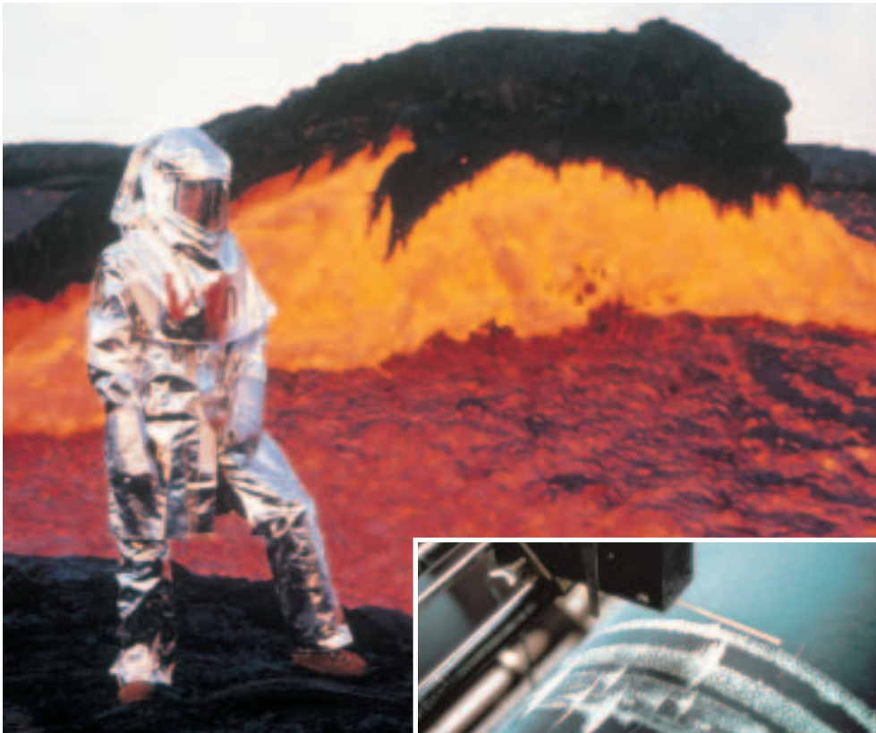
Figure 1.11 Geologists studying volcanoes must wear a special suit with a metal coating that reflects these intense temperatures. This allows them to get close enough to an eruption to make observations, take measurements, or collect gas and lava samples.
