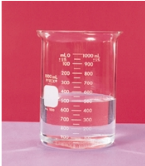
Figure 1.40 A solid object added to a container displaces the fluid.
