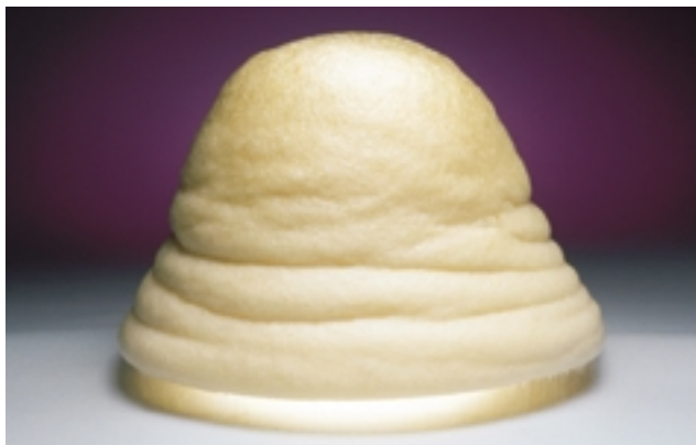
Figure 1.24 Thermoplastic polymers can be melted, “blown” full of air, and cooled to form a solid foam.
