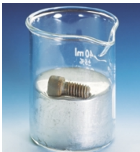
Figure 1.29 Liquid mercury is so dense that it can support a solid iron bolt. A layer of oil has been placed on top of the mercury to prevent vapour from escaping into the surrounding air.
