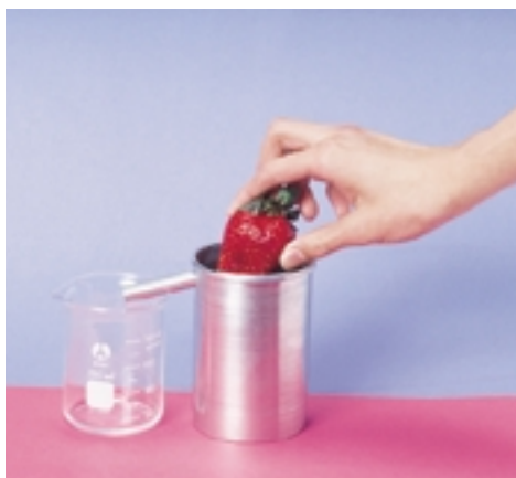
Figure 1.33 The volume of an irregularly shaped object can be found by measuring the volume of the water that spills out of an overflow can.
