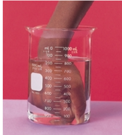
Figure 1.40 A solid object added to a container displaces the fluid.
