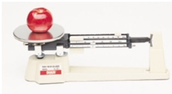
Figure 1.31 A balance is used to measure mass in grams (g) or in kilograms (kg). This apple has a mass of 102 g. It weighs about 1 N.
