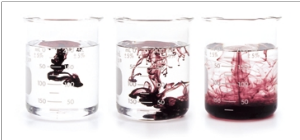
Figure 2.12 In time, the ink particles will become evenly dispersed with the water particles, and the whole solution will appear ink-coloured.
