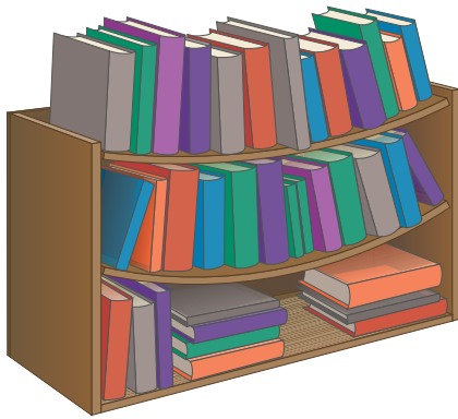
Figure 2.12 The force of gravity pulls down on the bookcase and the books. This is the load the bookcase must bear. This bookcase appears to be overloaded.
