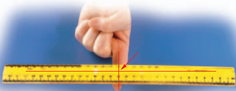
Figure 2.10 Try balancing a ruler on your finger. Where do you have to place your finger so the ruler will not fall? That point on the ruler is the centre of gravity.
