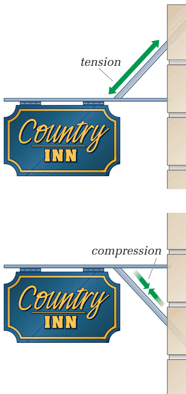
Figure 4.7 The component that provides support for the sign in (A) is called a “tie.” It works by resisting tension in the structure. The component that provides support for the sign in (B) is called a “strut.” It works by resisting compression in the structure.
