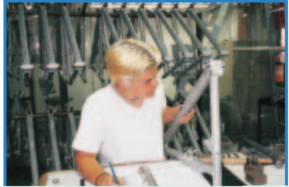
Figure 4.10 At Rocky Mountain Bicycles, the most important criteria for materials are strength, weight, and cost. Some of the materials that have the best strength-to-weight ratios are expensive and limited to only high-end (meaning high cost) bikes. Aluminum, which costs less, also has excellent strength-to-weight properties and is used to make mid- to high-end frames. Steel is generally used for mid- to low-end frames because of its low cost.
