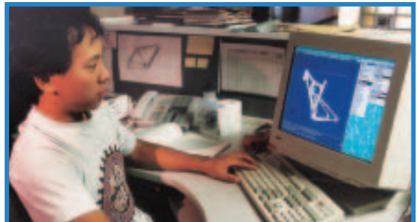
Figure 4.12 Rocky Mountain Bicycles uses computer-aided systems for all of its bike designing and manufacturing. This allows other departments in the company, such as marketing, to approve the design before an actual bike is built.
